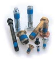
The NYLOK BLUE PATCH self-locking element is permanently spray bonded onto the threads of a fastener. When mating threads are engaged, the tough, resilient blue nylon patch element is compressed and a counterforce is created to establish a much stronger metal-to-metal contact and positive resistance to vibration and loosening.
