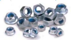
The NYLOK BLUE TORQ-PATCH LOCKNUT'S self-locking element is permanently spray bonded onto the threads of virtually any type nut. When mating threads are engaged, the tough, resilient blue nylon patch element is compressed and a counterforce is created to establish a much stronger metal-to-metal contact and positive resistance to vibration and loosening.
