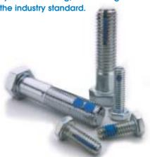
The NYLOK BLUE PELLET and TORQ-STRIP self-locking elements are permanently embedded in the threads of a fastener. When mating threads are engaged, the tough, resilient Blue nylon element is compressed and a counterforce is created to establish a much stronger contact and positive resistance to vibration and loosening.
