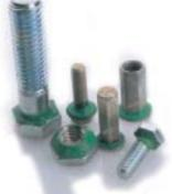
Green-colored **NYSEAL** creates a gasket-type seal, preventing leakage of fluids and gases under pressures up to 500 psi. The coating is permanently fused on the bearing surface of the fastener. As the screw is seated to its final position against the mating part, the **NYSEAL** element compresses slightly and fills the void under the bearing surface of the head and countersink/counterbore.
